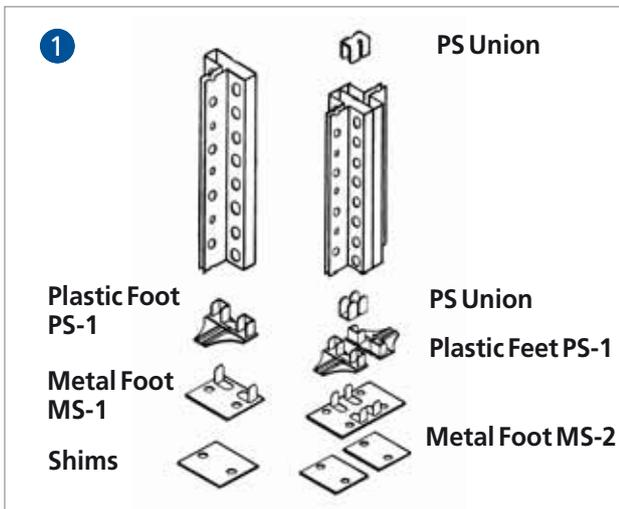
The lateral and interior sides of the uprights have slots every 25mm in order to facilitate the insertion of various components. The PS unions are designed to join two uprights when required. The metal feet fit into the lower ends of the uprights in order to reinforce their stability on the floor.
