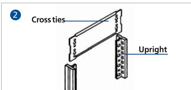
The cross ties are bolted to the uprights providing the shelving with transverse stability.
