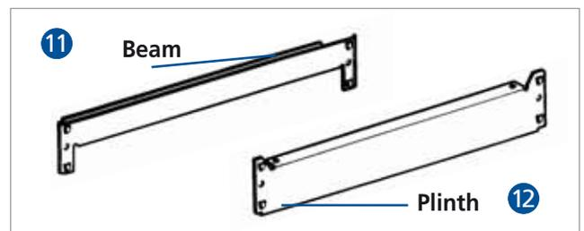
When cross bracing and back sheets are not used, the fitting of shelf beams will provide greater rigidity. In addition, shelf beams increase the loading capacity of the shelves.
