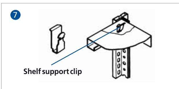
Shelves which are not supported by beams require four shelf support clips.
