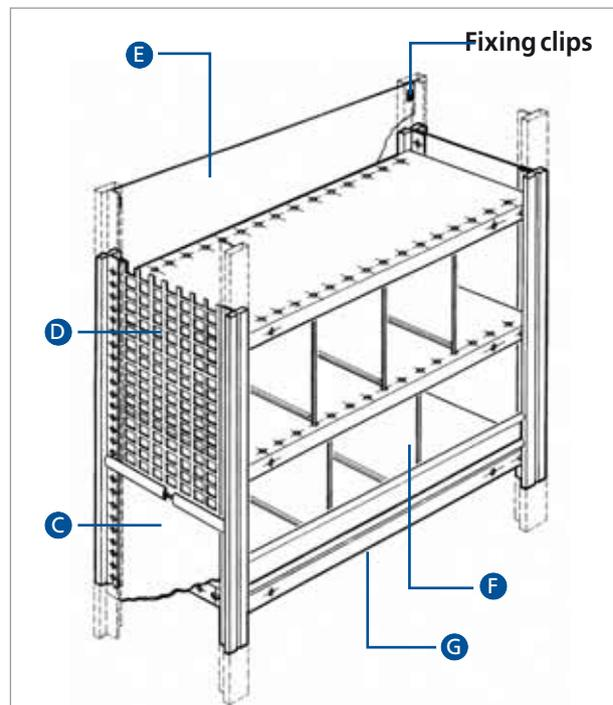
The fitting of lateral cladding (plain lateral sheet –C– , and perforated lateral sheet –D–), as well as the back sheets –E–, the slotted shelf dividers PR –F– and the shelf retainers –G– offer the possibility of creating closed compartments to ease the classification of items stored.
